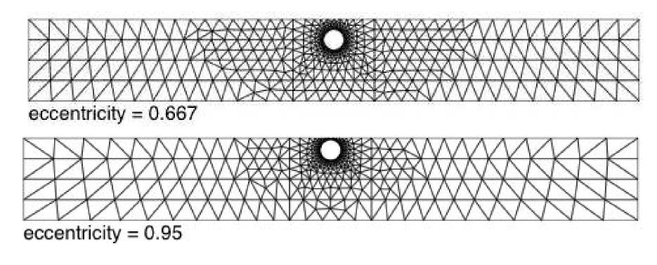
Figure 2: Mesh for pump flow in two dimensions.
