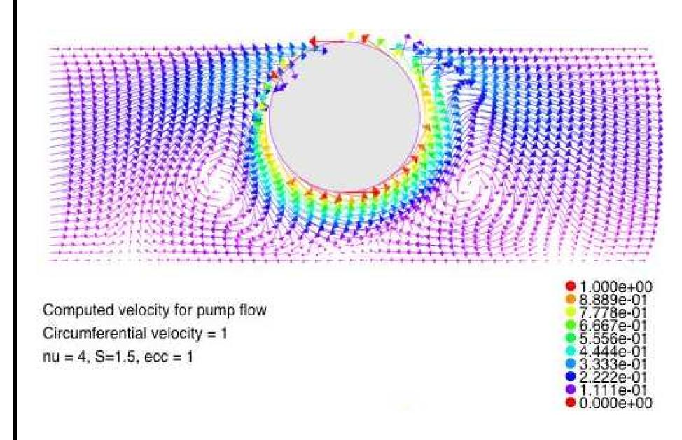
Figure 3: Pump flow in two dimensions
