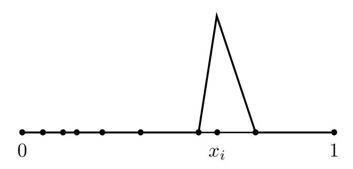
Figure 1: piecewise linear basis function  $\phi_i$
