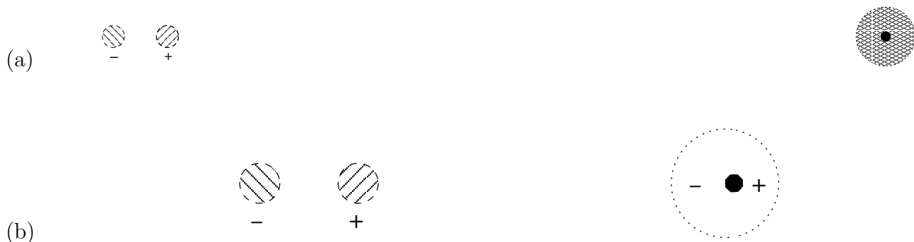
Figure 3.6: A dipole (left) inducing a dipole in a polarizable molecule (right). The upper configuration (a) shows the dipole and polarizable molecule well separated, and the lower configuration (b) shows them closer, with the molecule on the right now polarized.
