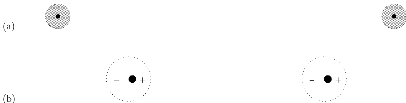
Figure 3.11: Mutual polarization of two molecules. The upper configuration (a) shows the polarizable molecules well separated, and the lower configuration (b) shows them closer, with the molecules now visibly polarized.
