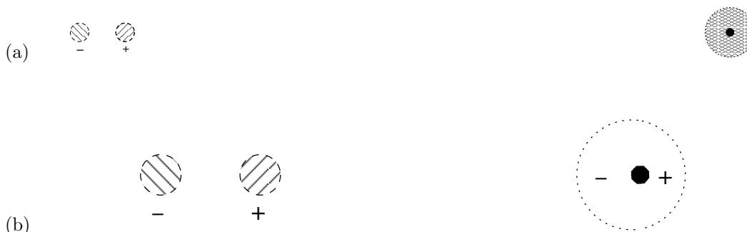
Fig. 3.10 The Debye force: a dipole (left) inducing a dipole in a polarizable molecule (right). The upper configuration (a) shows the dipole and polarizable molecule well separated, and the lower configuration (b) shows them closer, with the molecule on the right now polarized.
