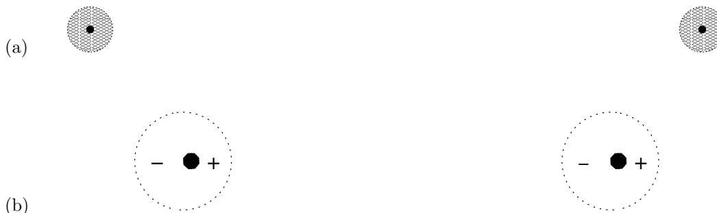
Fig. 3.11 Correlated polarization of two molecules. The upper configuration (a) shows the molecules well separated, and the lower configuration (b) shows them closer, with the electrons now visibly correlated.
