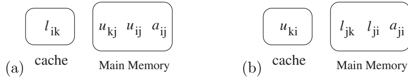
Figure 4.2: Residence of variables in cache and main memory in the compact scheme in the computation of line 1 (a) and line 2 (b) of (4.4).
