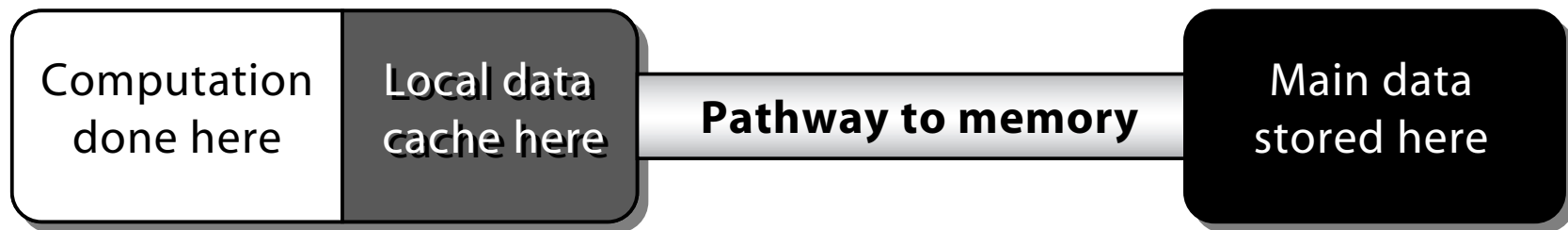
Figure 5: A memory model with a large local data cache separated from the main memory by a pathway with limited bandwidth \mu .
