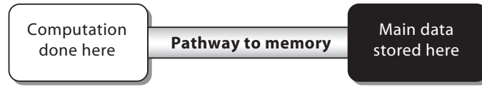
Figure 1.3 A simple memory model with a computational unit with only a small amount of local memory (not shown) separated from the main memory by a pathway with limited bandwidth \mu .
