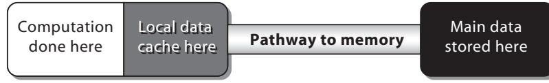
Figure 1.4 A memory model with a large local data cache separated from the main memory by a pathway with limited bandwidth \mu .
