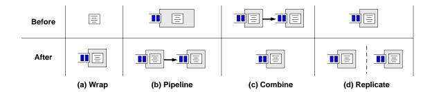
Figure 3: The Four Design Patterns: The four design patterns, wrap, pipeline, combine, and replicate, can be applied to stages of a service to condition it against load, failures, and limited or bottleneck resources.
