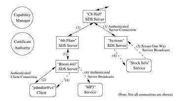
Figure 10: Components of the Berkeley SDS: Dashed lines correspond to periodic multicast communication between components, while solid lines correspond to one-time transport connections.
