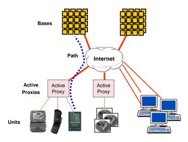
Figure 1: The Ninja Platform Architecture: The architecture consists of bases (services running on clusters of workstations), active proxies (stateless or soft-state intermediaries between units and services), units (heterogeneous devices and sensors), and paths (a composition chain across units, proxies, and services in bases).
