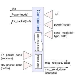
Figure 9: A TinyOS Software Component: Each TinyOS software component accepts and emits commands and events. Commands flow from higher level layers to lower levels, and events flow from lower level layers to higher levels.
