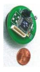
Figure 8: A TinyOS-based Mote: This "mote" includes a 4MHz microcontroller, a software-driven radio, and an application that coordinates with neighboring motes to discover an ad-hoc sensor network routing topology.
