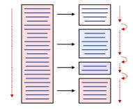
Figure 2: **Splitting a Service into Stages**: Our programming model views a service as a sequence of stages, separated by high-or variable-latency operations. Stages only share data using pass-by-value semantics, for example, by exchanging messages.
