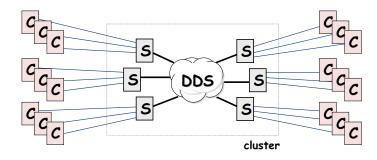
Figure 5: **High-level view of a DDS:** A DDS is a self-managing data repository running on a cluster of workstations. All service instances (S) in the cluster see the same consistent image of the DDS; as a result, any WAN client (C) can communicate with any service instance.
