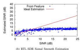
Fig. 5. Estimating the signal strength of a legitimate user from its feature strength.
