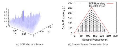
Fig. 1. Building and encoding cyclostationary features. (a) A cyclostationary feature at ( $\alpha=64$ , k=102). (b) A sample feature constellation map for transmitters with  $\alpha$  resolution = 4 and k resolution = 10 (FFT = 256, CP length = 64), mapping to 9 bits per feature.
