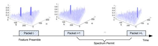
Fig. 2. Each Gelato permit consists of its feature preamble and a group of features carrying the permit bit stream. The preamble carries two features, one on each half of the k-axis, carrying information on the FFT size and CP length required to decode the subsequent feature packets.
