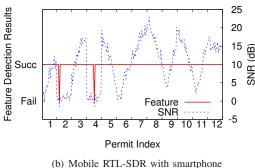
Fig. 4. Impact of mobile police nodes. When walking around a large  $12m \times 7m$  room with a Gelato receiver, we observe very few feature decoding errors caused by deep channel fades.
